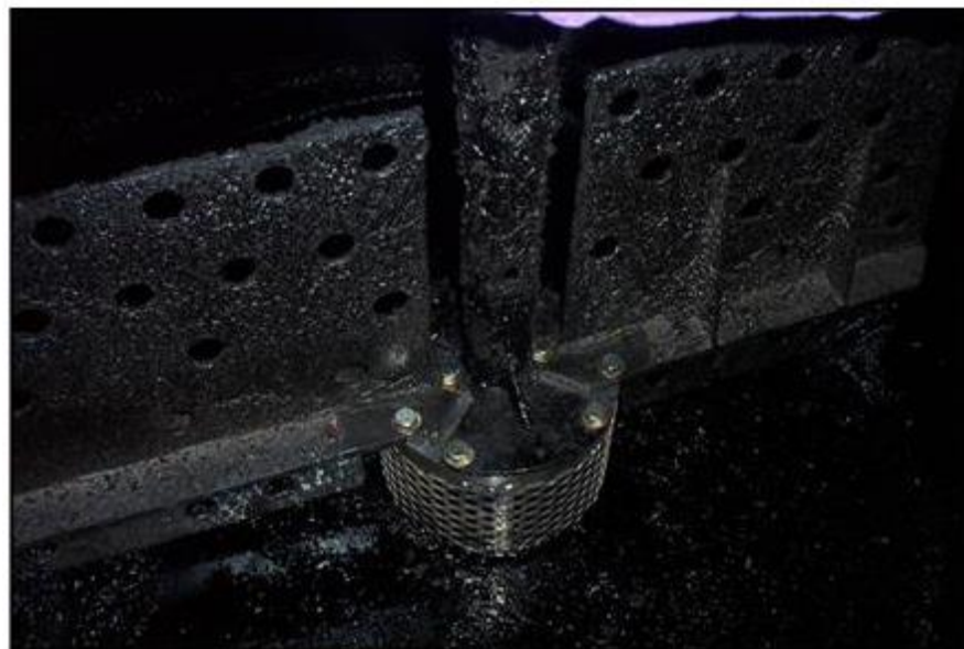
Figure 6-11 Agitator Shaft and Paddle Mounting
