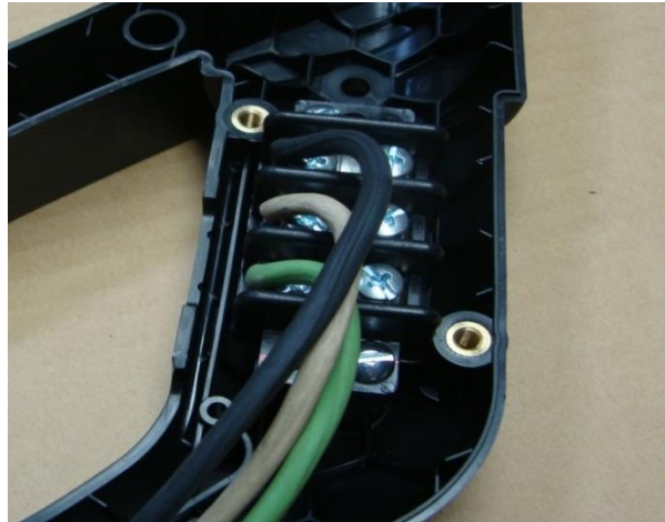
Figure 6-18 Terminal Block Wiring
