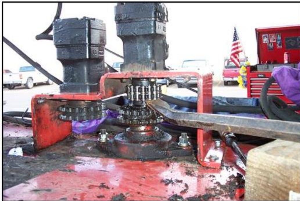
Figure 6-13 Pump Shaft to Hydraulic Motor Placement
