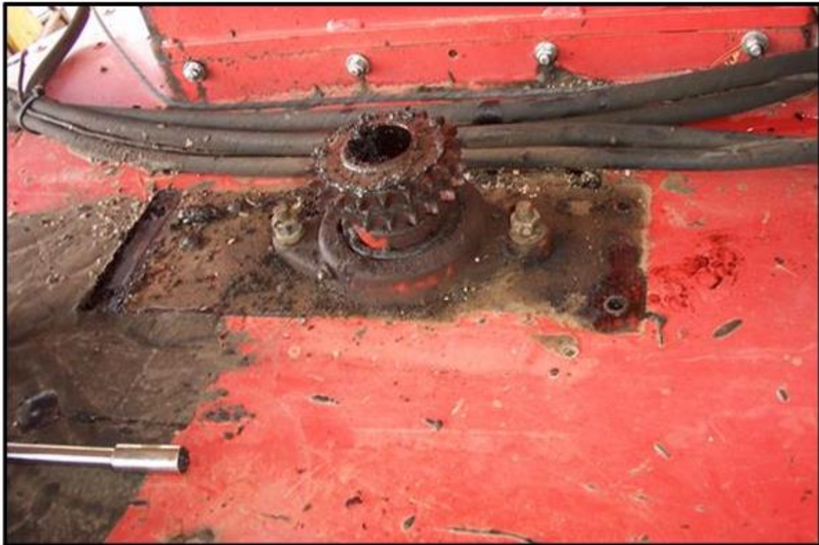
Figure 6-5 Removal of Motor Mount Assembly
