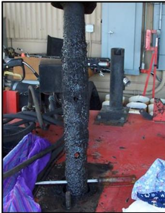
Figure 6-6 Supporting the Agitator Away from the Material Pump
