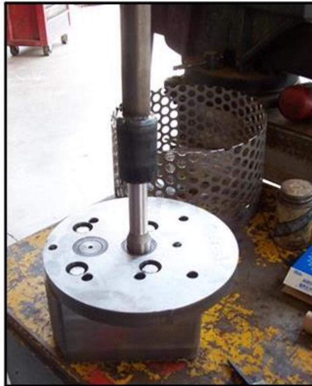
Figure 6-9 Pump Drive Shaft Dry Fit to Material Pump
